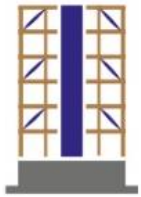
26) Podium, core, and steel bracing
